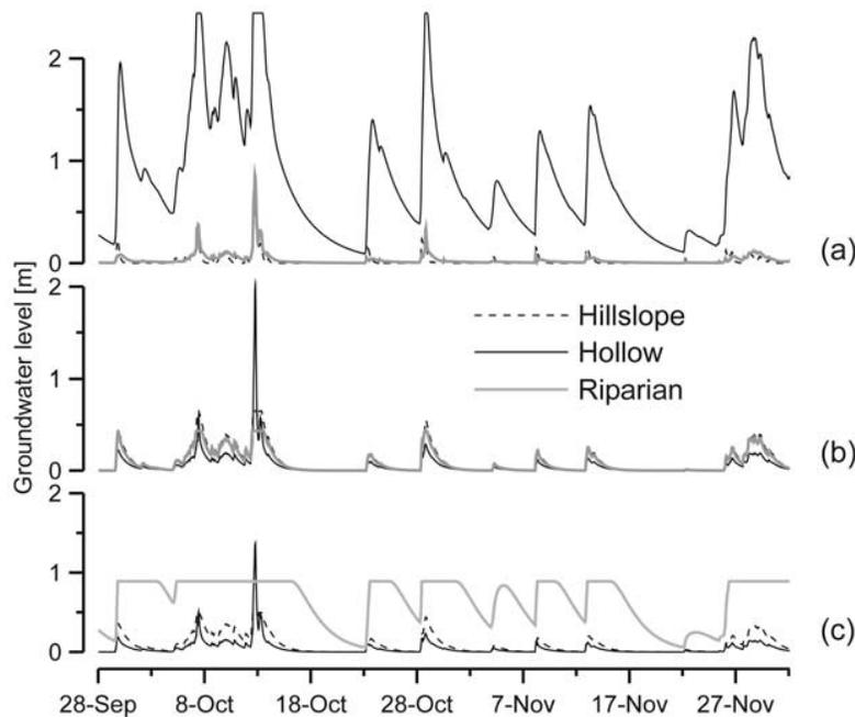
**Figure 5.** Three model runs with different parameter sets resulting in different groundwater dynamics. All three parameter sets had been calibrated to observed runoff and gave an almost similar goodness of fit (model efficiency  $\sim 0.93$ ). None of the three sets of groundwater time series agrees with the perceptual model of the watershed.
