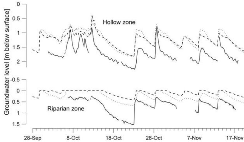
**Figure 7.** Comparison of groundwater level simulations (dashed line) for the riparian and the hollow box and levels extracted from tensiometer observations (solid line) (levels are here given in m below ground surface). The dotted line shows the simulated groundwater levels when using the alternative goodness of fit criteria.
