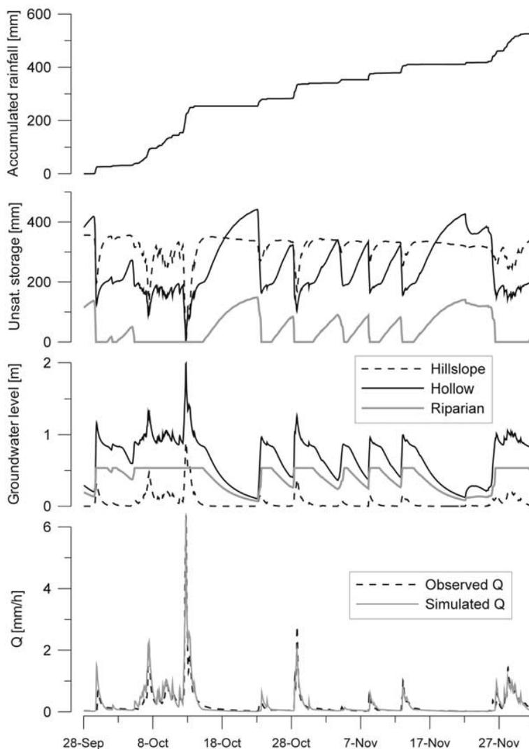
**Figure 6.** Simulation with best overall performance. Accumulated rainfall, simulated unsaturated storage, and simulated groundwater levels (m above bedrock) as well as observed and simulated runoff. The model efficiency for runoff is 0.84, and the simulated groundwater dynamics agree in general with the perceptual model.
