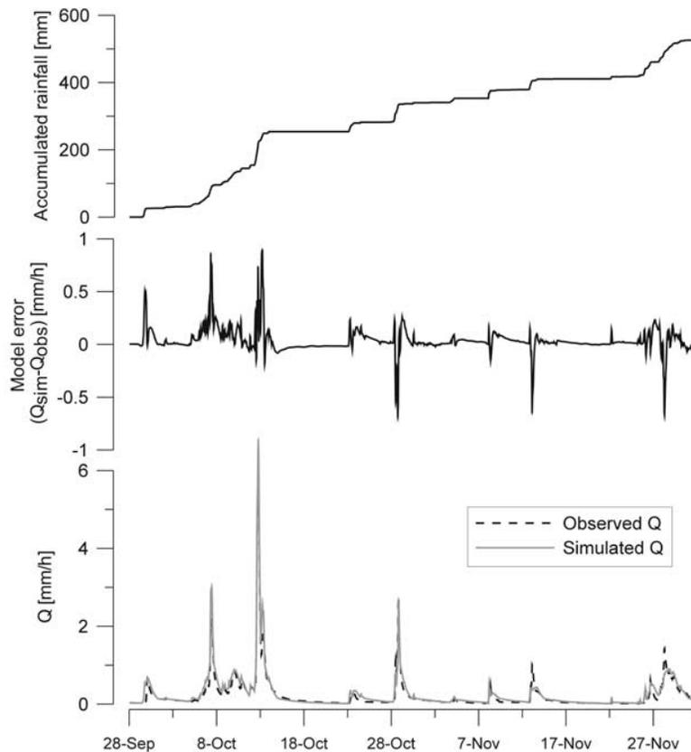
**Figure 3.** Accumulated rainfall, runoff model error, and observed and simulated runoff for the period September–December 1987. Measured data are shown as dashed line. The simulation of runoff (solid line) is based on the calibration using only runoff data.
