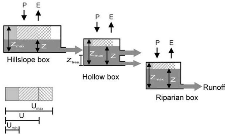
**Figure 1.** Structure of the three-box model developed for the Maimai M8 watershed including hillslope, hollow, and riparian zone reservoirs. P, precipitation; E, evaporation;  $z$ , groundwater level above bedrock;  $z_{max}$ , maximal groundwater level above bedrock;  $U$ , unsaturated storage.
