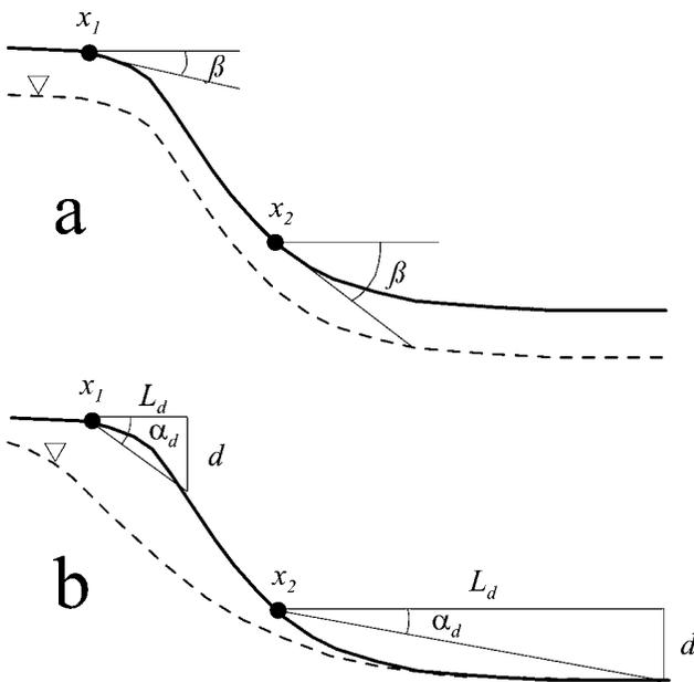
**Figure 1.** A drawing of a hillslope flow path in profile that illustrates the differences between (a) the local gradient ( $\tan\beta$ ) and (b) the downslope index ( $d/L_d$  or  $\tan\alpha_d$ ) for points  $x_1$  and  $x_2$ . The groundwater table in each plot is assumed to reflect the calculated gradients.
