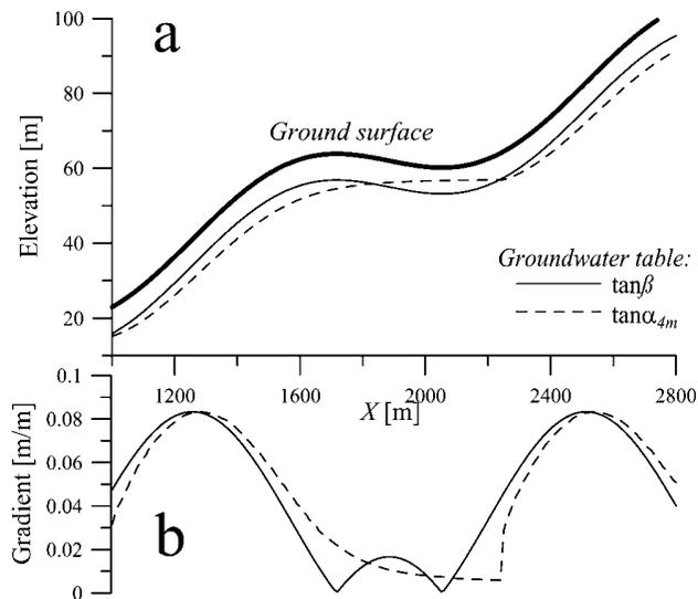
**Figure 2.** Local gradient,  $\tan\beta$ , and the downslope index,  $\tan\alpha_{d,m}$ , calculated for a computer-generated hillslope profile. (a) Approximate groundwater table elevations were calculated from (b) the gradient data to better illustrate the differences. A groundwater table depth of 6 m at  $X=2250$  m was assumed as the starting point for this integration.
