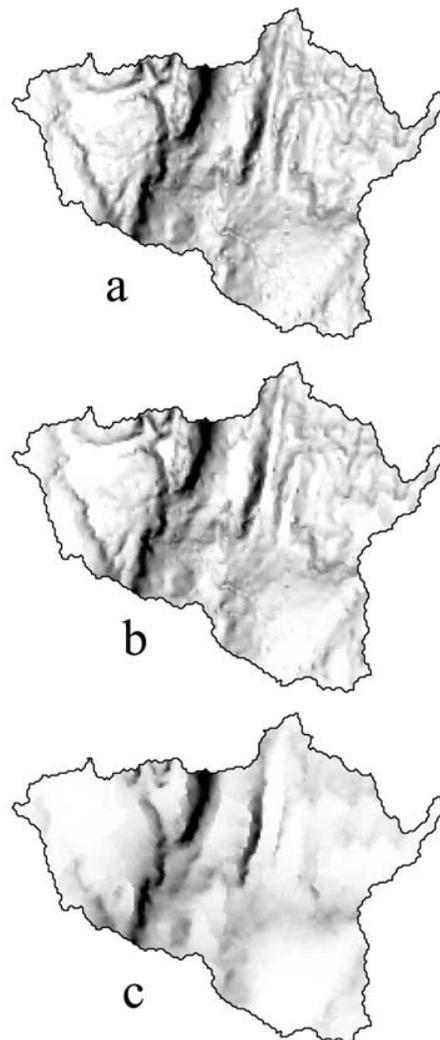
**Figure 3.** Raster coverages of (a)  $\tan\beta$ , (b)  $\tan\alpha_{2m}$ , and (c)  $\tan\alpha_{10m}$  for the 41 ha W-9 catchment at Sleepers River, Vermont. Steep gradients are dark in the figures.
