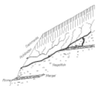
**Figure 1.** The original perceptual model of subsurface stormflow by Engler 1919. The hatched areas represent the uniform infiltration of water in the humus (*Dammerde*) and the soil (*Rohboden*). Deeper in the profile, water is flowing in “veins” laterally. *Nagelfluh* is the bedrock type for a specific geological setting in Switzerland
