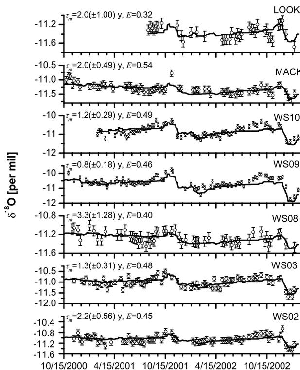
**Figure 4.** Measured and simulated  $\delta^{18}O$  for each catchment using exponential residence time distributions. The estimated mean residence times ( $\tau_m$ ) are shown with 95% confidence limits ( $2\sigma_p$ ) in parentheses, and Nash-Sutcliffe efficiency measures ( $E$ ) [Nash and Sutcliffe, 1970] are shown for model simulation comparisons. Error bars indicate the analytical reproducibility for  $\delta^{18}O$  measurements.
