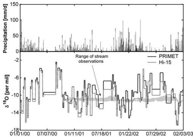
**Figure 2.** Daily precipitation and weekly  $\delta^{18}\text{O}$  measured at PRIMET (430 m) and Hi-15 (922 m) meteorological stations. The shaded area shows that range of measured streamflow  $\delta^{18}\text{O}$  for all catchments.
