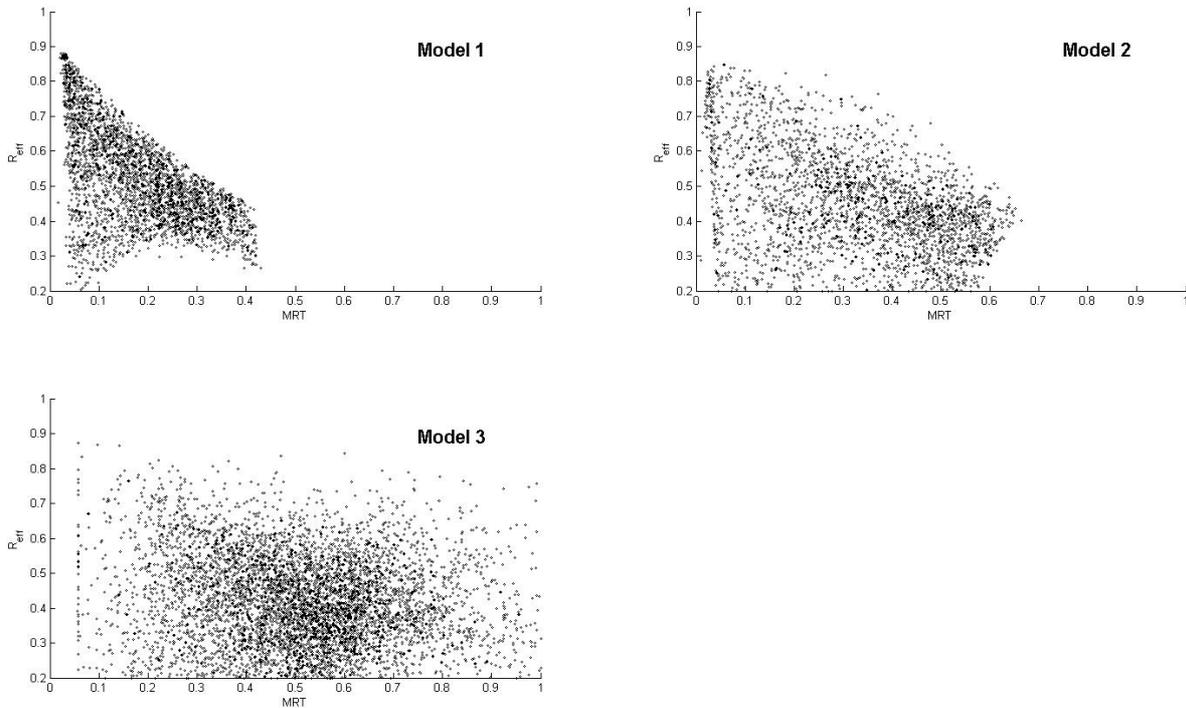
**Fig. 2** Scatter plots of discharge versus MRT efficiencies for the 3 models. Discharge efficiency is the Nash-Sutcliffe statistic and MRT efficiency is reported as the ratio of the modelled value to the measured value (120 days). Some values of MRT efficiency were greater than 1, and the bottom axis is truncated for clarity.
