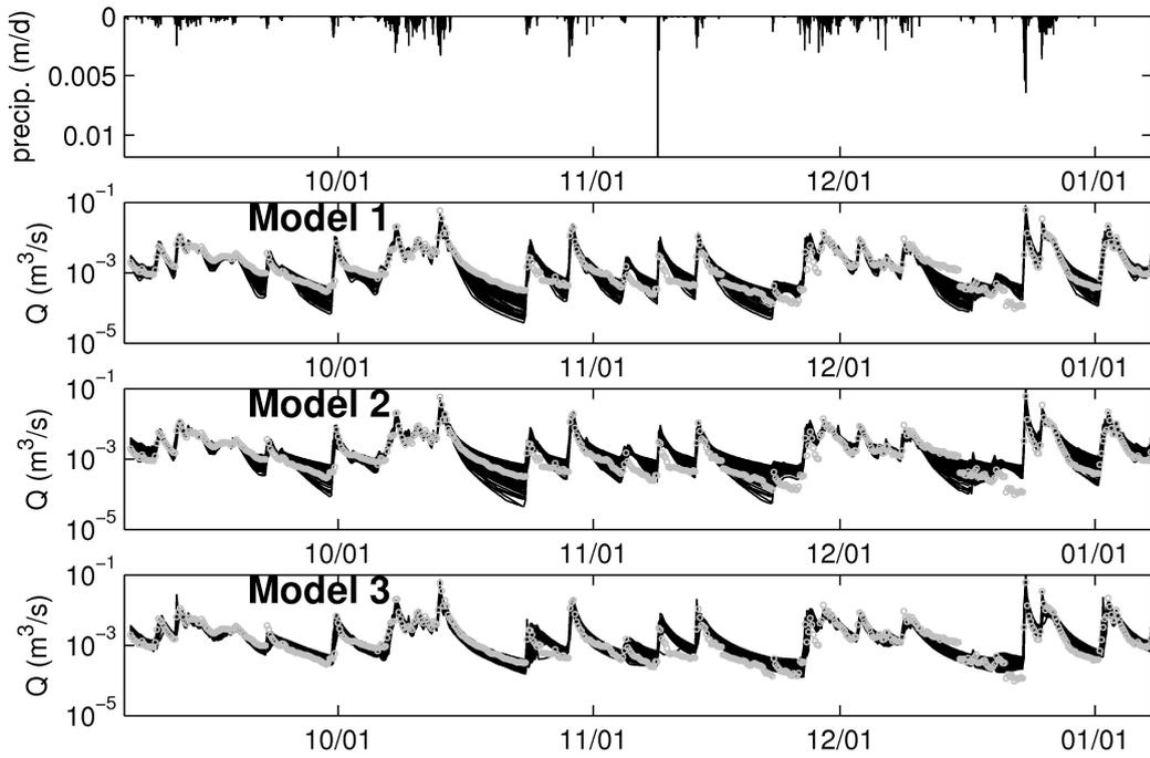
**Fig. 1** Simulation results for stream discharge. The Y axis is log transformed to outline more clearly model results at lower discharge. The calibration strategy focused on untransformed  $R_{eff}$ , and peak flows are correspondingly better captured. The plotted simulations are those found with Nash-Sutcliffe efficiencies over 0.75. Measured values are plotted as crosses.
