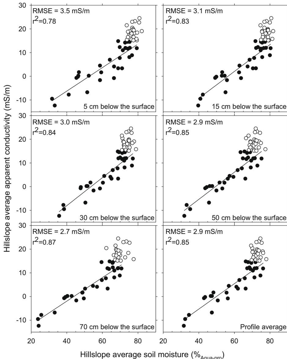
**Fig. 2.** The linear relation between hillslope average apparent conductivity (9.090 kHz) below the threshold (15 mS/m for 9.090 kHz) and hillslope average soil moisture at different depths below the surface. Conductivity values below the threshold are shown with solid circles while the conductivity values above the threshold are shown with open symbols. Relationships for the 7.290, 11.250, 14.010 kHz frequencies are similar to the results shown here for the 9.090 kHz frequency.
