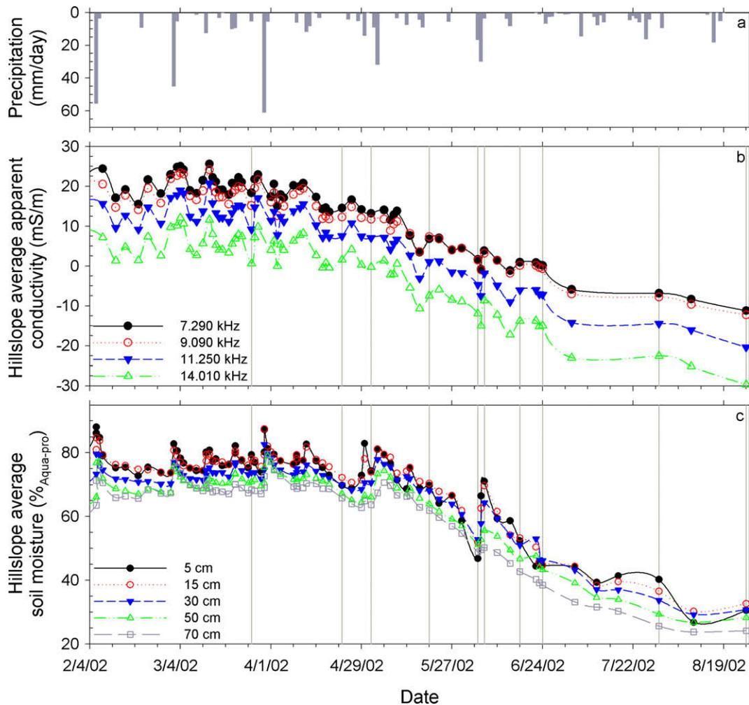
**Fig. 1.** Time series of daily precipitation (a), hillslope average apparent conductivity measured by the four frequencies (b), and hillslope average soil moisture at different depths below the surface (c). The vertical gray lines represent the times of the spatial soil moisture maps shown in Fig. 6.
