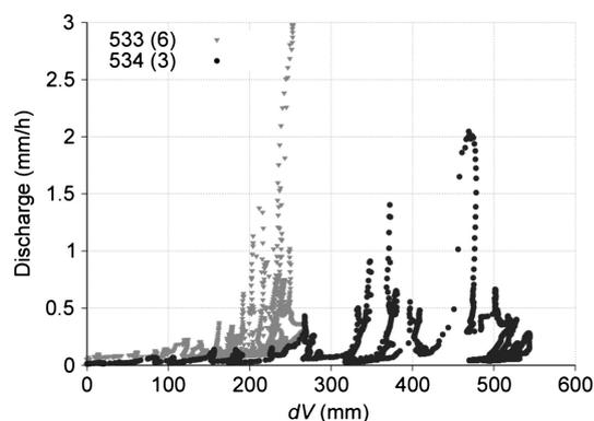
Figure 4. The relationship between change in total storage  $dV$  and discharge  $Q$  from two sub-watersheds. Both watersheds have almost no runoff response when the  $dV$  values are below 200 mm at no. 533 watershed (6 km<sup>2</sup>) and 350 mm at no. 534 (3 km<sup>2</sup>), respectively. At the no. 533 watershed, the  $dV$  plateaus around the 200- to 250-mm level, whereas at the no. 534 watershed, the  $dV$  increases gradually even after runoff activation, and finally, it exceeds 500 mm
