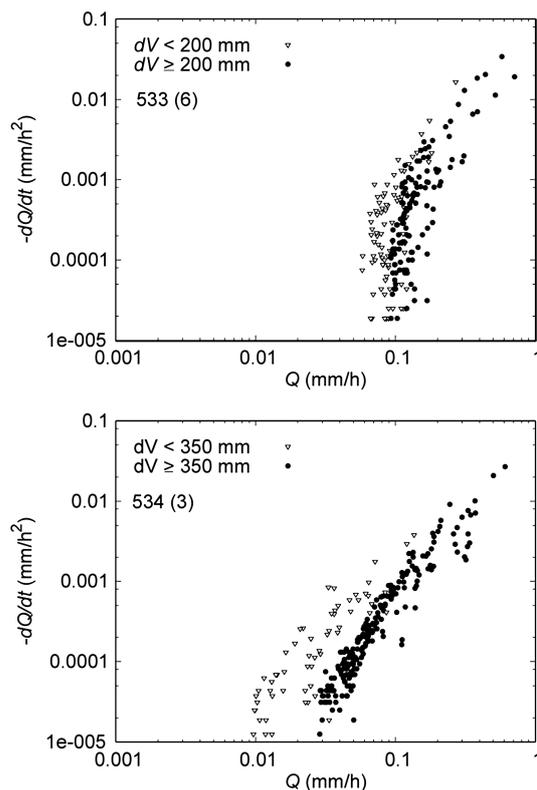
Figure 6. The relationship between recession rates ( $-dQ/dt$ ) and runoff  $Q$  from two sub-watersheds (nos. 533 and 534). The plots are classified into two groups based on the  $dV$  values ( $dV=200$  mm and  $dV=350$  mm were used as the thresholds to distinguish before and after wet-up)
