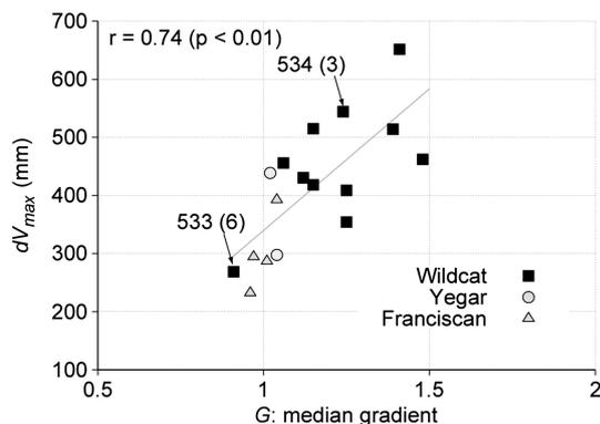
Figure 5. The relationship between median gradient  $G$  for each sub-watershed and its maximum total storage change ( $dV_{max}$ ) during the rainy season. The symbols represent the three basic geologic units that comprise the overall watershed area
