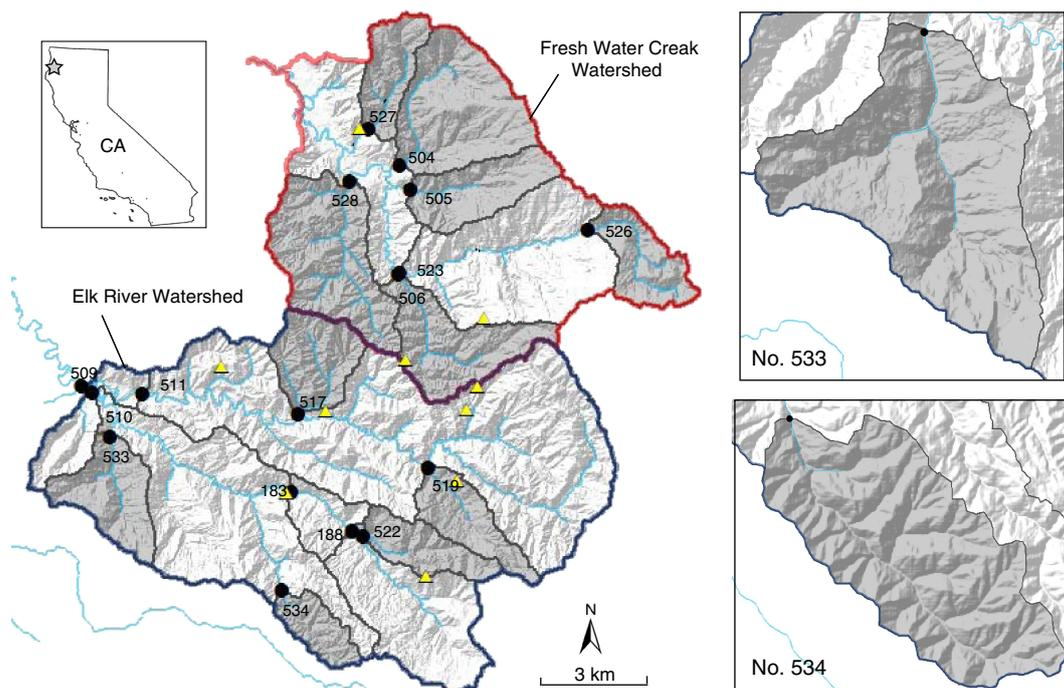
Figure 1. Map of Elk River watershed ( $110\text{ km}^2$ ) and Freshwater Creek watershed ( $76\text{ km}^2$ ). The black dots represent the 17 discharge gauging stations, and the triangles represent the ten rain gauges in the two adjacent watersheds
