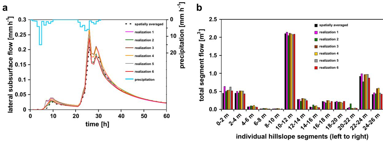
Fig. 4. Comparing subsurface stormflow response for the six forest realizations and spatially averaged throughfall. (a) Subsurface stormflow hydrographs. (b) Spatial distribution of subsurface flow along the downslope boundary of the hillslope, showing total subsurface flow per 2 m segment for the scenarios (from left to right facing upslope).
