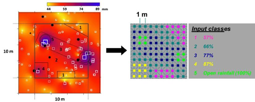
**Fig. 2.** Discretizing the interpolated throughfall map by Keim et al. (2005) (left; see their (c)) into five input classes that were used as surface boundary conditions in the simulations. Open white squares in Keim et al.'s figure indicate throughfall collectors, scaled to storm-total throughfall. The underlying color pattern was derived by interpolation by Kriging parameterized from variograms (see Keim et al. (2005) for more details on methods).
