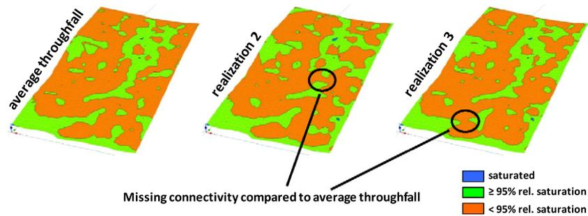
**Fig. 10.** Saturation patterns (as relative saturation) at the soil–bedrock interface at 4 h before the end of the storm, shown for three scenarios (first set of simulations). The general pattern reflects the bedrock topography (see Fig. 1).
