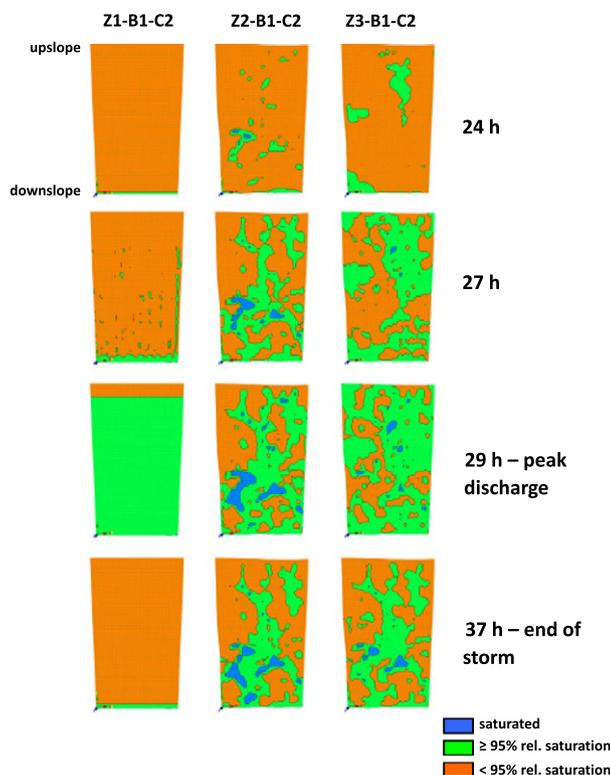
**Fig. 9.** Saturation patterns (as relative saturation) at the soil–bedrock interface for the three hillslope geometries (spatially averaged input, natural storm) at four time steps during the storm event (second set of simulations). See Fig. 7 for corresponding hydrographs and Fig. S2 in the Supplementary information for plots showing pressure head  $h$  along the downslope boundary for the soil–bedrock interface for time step  $t = 29$  h.
