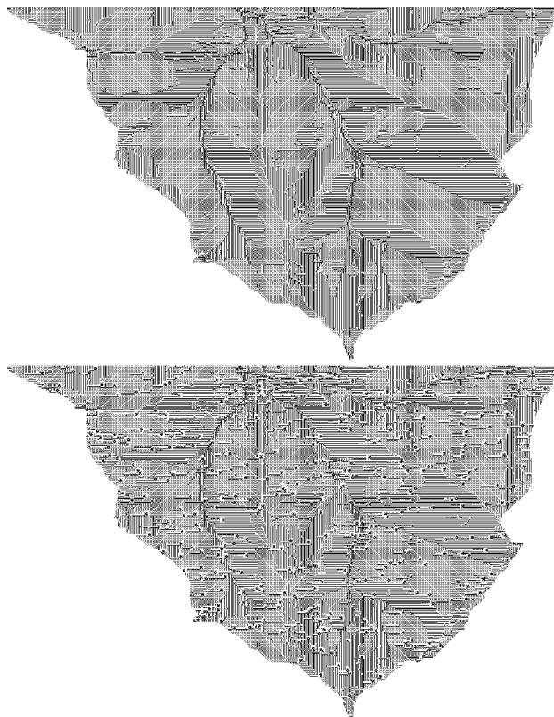
Figure 8. Drainage network with all depressions removed from the DEM (1 m × 1 m) without any tree throw (Baseline) (top) and after a tree-throw event with pits, mounds and tree trunk (Pit–Mound–Tree) randomly distributed. Only the top one third of the catchment is shown for clarity. Catchment outlet at the top of each image.
