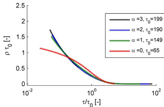
**Fig. 4.** Effect of rate of exponential decline in  $k_s$  with soil depth ( $\alpha$ ) on dimensionless TTD.  $\tau_0$  represents mean groundwater age (day). The Gamma shape parameter of the TTD varies from 0.92 to 0.50 as  $\alpha$  increases from zero to 3.
