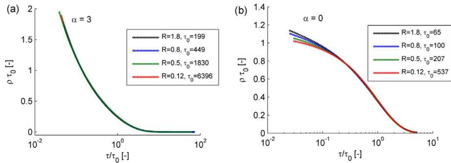
Fig. 8. Effect of infiltration rate ( $R$  [mm/d]) on dimensionless transit time distribution for two different rates of exponential decline in  $K_s$  with depth ( $\alpha$ ). (a)  $\alpha = 3$  (extreme heterogeneity), the Gamma shape parameter varies from 0.52 to 0.50 as  $R$  increases from 0.12 to 1.8 mm/d. (b)  $\alpha = 0$  (homogenous case), the Gamma shape parameter varies from 0.97 to 0.92 as  $R$  increases from 0.12 to 1.8 mm/d.
