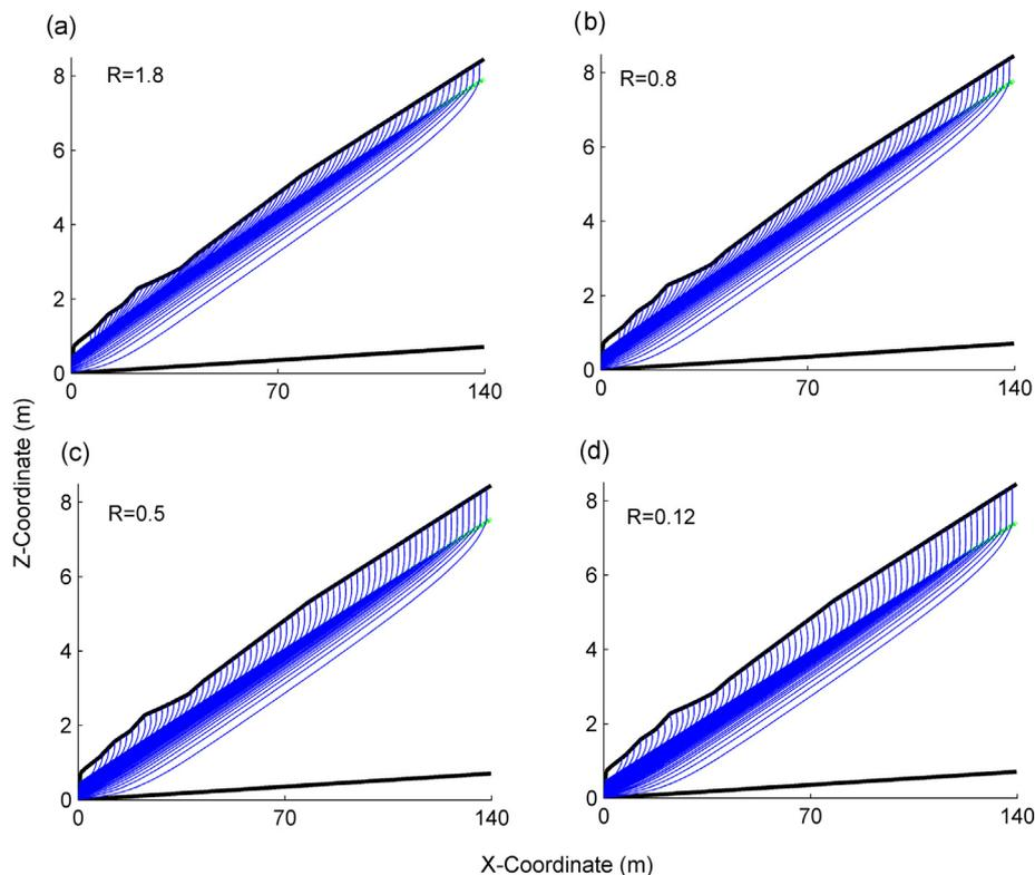
**Fig. 6.** Flow pathline distribution and water table (green line) for different values of infiltration rate ( $R$ ). (a)  $R = 1.8$  mm/d (high flow), (b)  $R = 0.8$  mm/d (average flow), (c)  $R = 0.5$  mm/d (median flow) and (d)  $R = 0.12$  mm/d (low flow). Only  $\frac{1}{8}$  of all particles used in the RWPT analysis were shown. (For interpretation of the references to color in this figure legend, the reader is referred to the web version of this article.)
