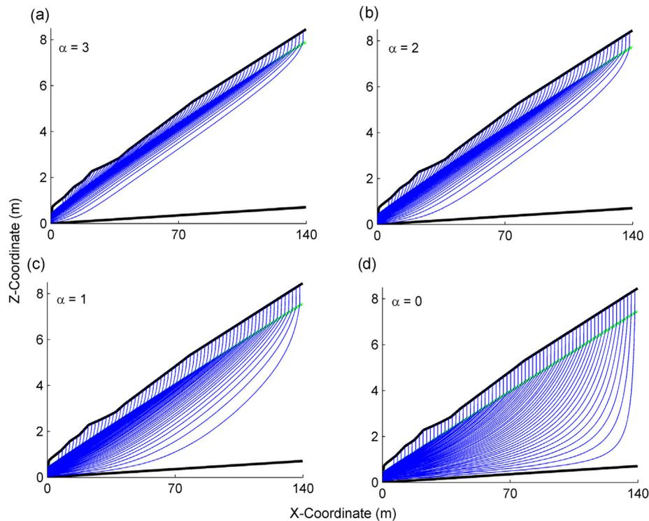
**Fig. 3.** Flow pathline distribution and water table (green line), for different rates in the exponential decline of  $k_s$  with soil depth ( $\alpha$ ). (a)  $\alpha = 3$ , (b)  $\alpha = 2$ , (c)  $\alpha = 1$  and (d)  $\alpha = 0$  (homogenous case). Only  $\frac{1}{8}$  of all particles used in the RWPT analysis were shown. (For interpretation of the references to color in this figure legend, the reader is referred to the web version of this article.)
