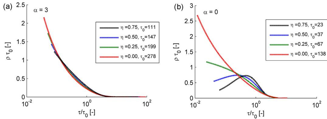
**Fig. 5.** Effect of the strength of exponential decline in porosity with depth ( $\eta$ ) on the dimensionless transit time probability density function.  $\tau_0$  represents mean groundwater age (day). (a)  $\alpha = 3$  (extreme vertical heterogeneity in  $K_s$ ), the Gamma shape parameter varies from 0.43 to 0.66 as  $\eta$  increases from 0 to 0.75. (b)  $\alpha = 0$  (homogenous  $K_s$ ), the Gamma shape parameter varies from 0.63 to 1.70 as  $\eta$  increases from 0 to 0.75.
