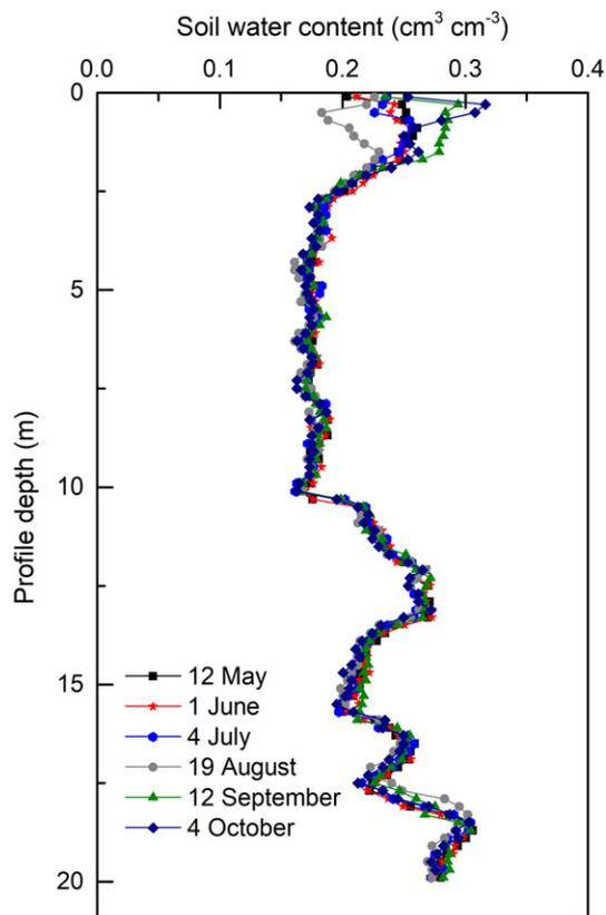
**FIGURE 2** In-situ neutron probe measured soil water contents (SWCs) in the “15-year”-old orchard in the 2017 growing season (in 2017, the trees are 16 years old)
